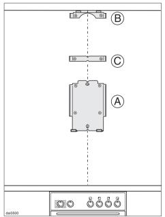
The ventilation system will be mounted to the wall through the use of retaining plates. Plate A is installed first, followed by plate B. Plate C should only be used if the distance between plate A and plate B is greater than 14 <sup>3</sup>/<sub>8</sub>" (365 mm).
